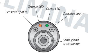
Setting the device is done after its installation by touching the magnetic pen to sensitive spots — and +. The setting process is indicated by the orange LED "STATE". Connect the level meter to the power supply. Using a measuring device or associated device, check its output - current or voltage.
