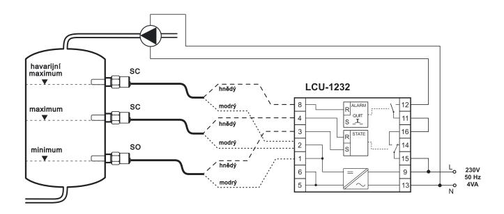
Pumping control with ALARM function detecting emergency minimum Connection with sensors with SO, SC output (e.g. GPLS-25N, CLS-18)
