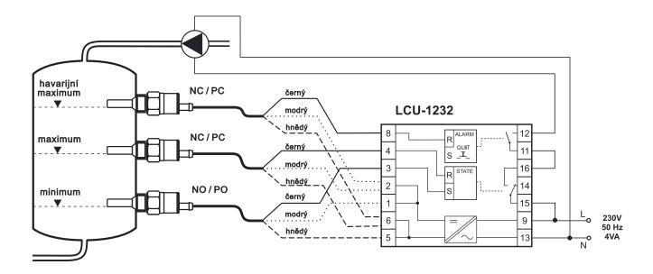
Pumping control with ALARM function detecting emergency minimum Connection with sensors with NPN or PNP output (e.g. DLS-27N, CPS-24N)
