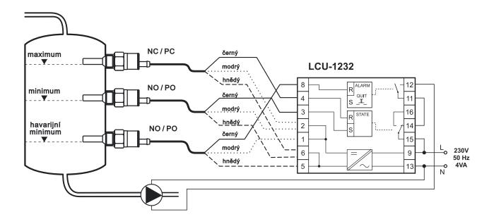
• Pumping control with ALARM function detecting emergency maximum Connection with sensors with SO, SC output (e.g. GPLS-25N, CLS-18)
