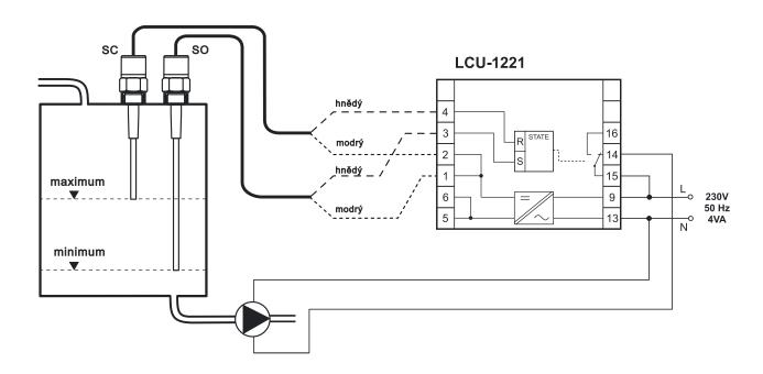
• Regulation by pumping. Connection with sensors with SO, SC output (e.g. GPLS-25N, CLS-18).
